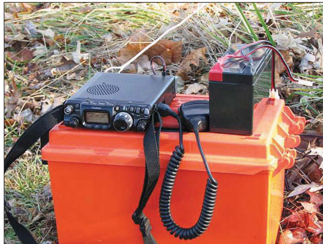
Figure 3 — Self contained station using a zip cord antenna and feed line.
