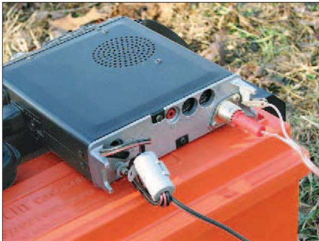
Figure 2 — Rear of radio showing banana plug and clip lead connections.
